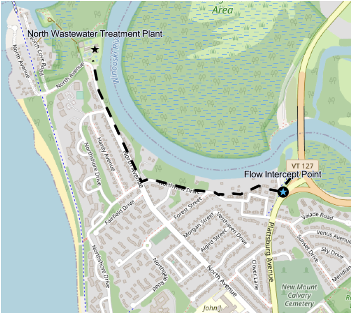
This photo shows the temporary on-ground sewer alignment as well as the location of North Plant and the flow interceptor point.
