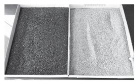
Filter sand cleaning and replenishment for FY18. 6 out of the 8 filters are complete. Above picture shows the sand before cleaning and right picture—after the cleaning."
