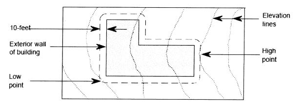
2. From the highest and lowest finished grade elevation points identified, average the two elevation points to establish the starting point for measuring building height.
