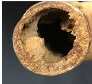
The photos above depict failed galvanized service lines in Burlington.
