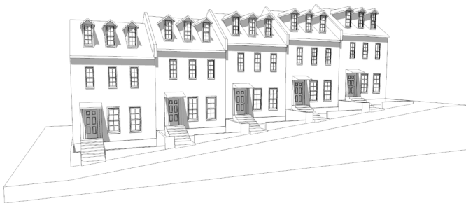
Illustration 14.6.4-A - Appropriate Site Grading
