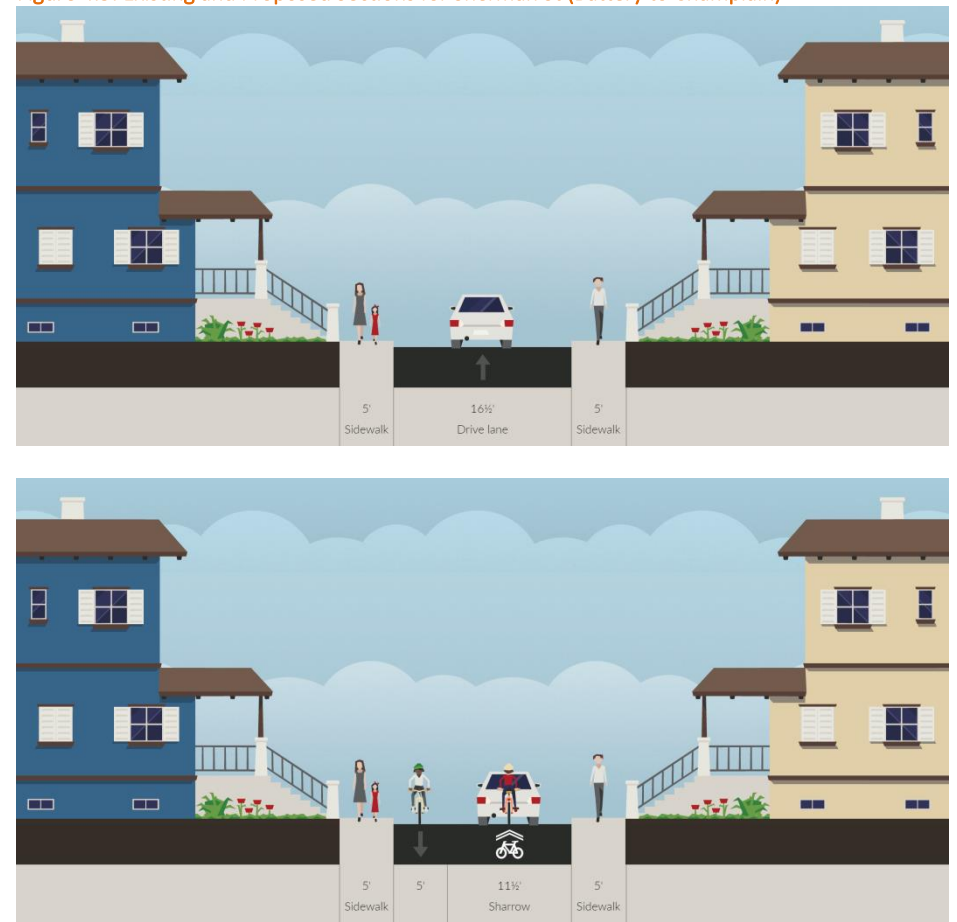
Figure 4.5: Existing and Proposed Sections for Sherman St (Battery to Champlain)
