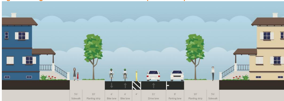
Figure 8: Long Term Cross Section for North Champlain Bikeway
