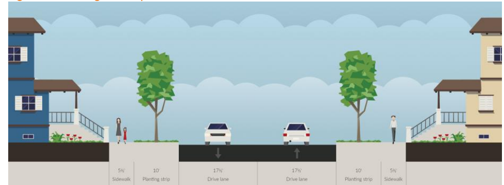
Figure 4.9: Existing and Proposed Sections: Elmwood from Peru to Grant
