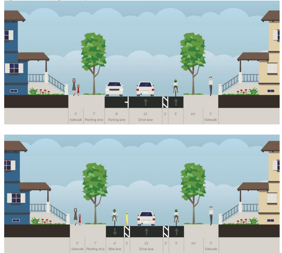
Figure 4.10: Existing and Proposed Cross Sections: North Union from Grant to Loomis
