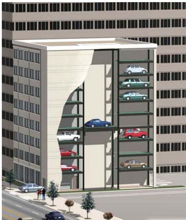
Figure 7: Automated Parking System with Access from Bottom (source: Robotic Parking)
