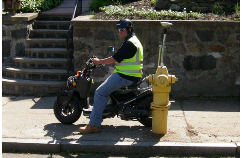
The Mapping Scooter on the sidewalk taking GPS coordinates of a hydrant
