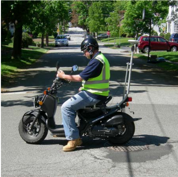
The Mapping Scooter taking GPS coordinates of a manhole
