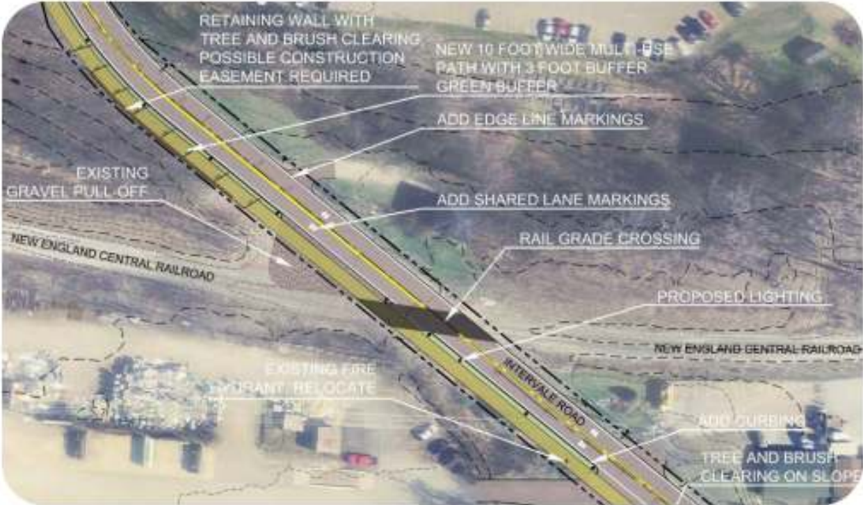
Figure 12: CAD Sketch of the Preferred Alternative at New England Central Railroad Crossing
