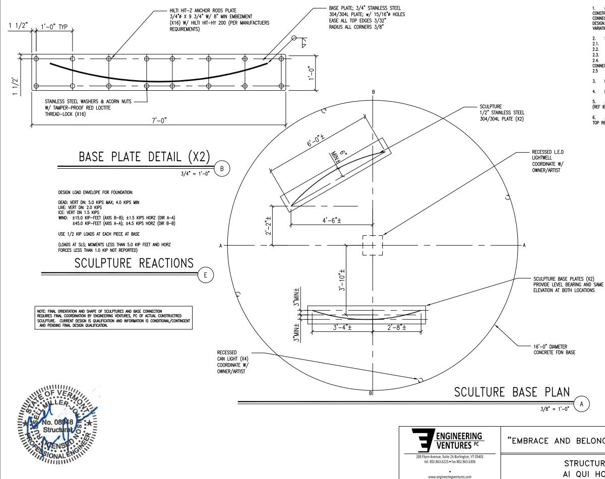
1. OVERALL STRUCTURAL SHAPE OF BASE AND SCULPTURE MAY VARY PENDING FINAL CONSTRUCTION BY ARTIST. FINAL DESIGN REQUIREMENTS FOR SCULPTURE AND CONNECTION AT BASE IS CONTINGENT ON A REVIEW OF FINAL SHAPE. FOUNDATION DESIGN SHALL ALSO ACCOMMODATE A TOLERANCE IN LOAD AND LOCATION FOR MINOR VARIATIONS AND A FINAL REVIEW.
