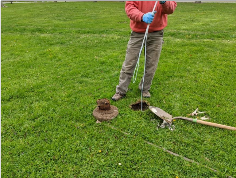
Photo #1: Removing dedicated LDPE tubing from well after prying out box.
