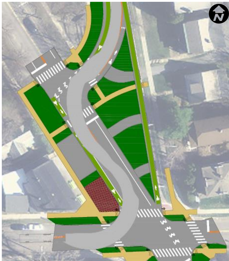
FIGURE 4-7: SOUTHBOUND S. WINOOSKI AVE. BURLINGTON LADDER TRUCK MANEUVERING TO WESTBOUND HOWARD ST.
