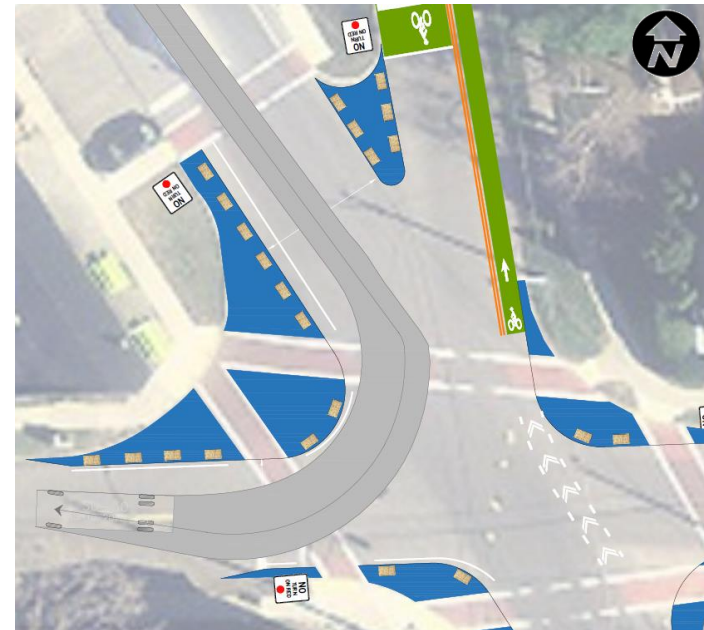
FIGURE 4-3: SOUTHBOUND SU-30 VEHICLE TURNING RIGHT ONTO WESTBOUND HOWARD STREET
