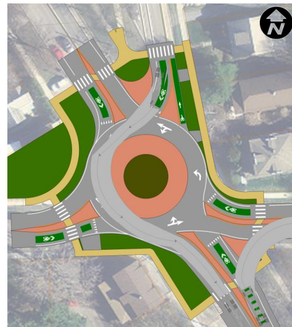
FIGURE 4-12: A SU-40 TRUCK (LARGER THAN THE DESIGN VEHICLE) NAVIGATING THE ROUNDABOUT
