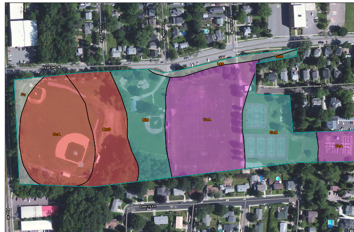
Map (left) Natural Resource Conservation Service (NRCS) Map of Calahan Park. These maps can help initiate the study of park soil characteristics that is critical to effective stormwater infiltration.
