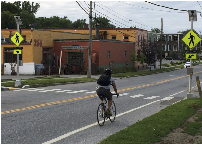
Figure 3-3: Rectangular Rapid Flashing Beacons were recently installed along Pine Street at pedestrian crossings and a 5' bike lane is provided along the south bound lane of the road.
